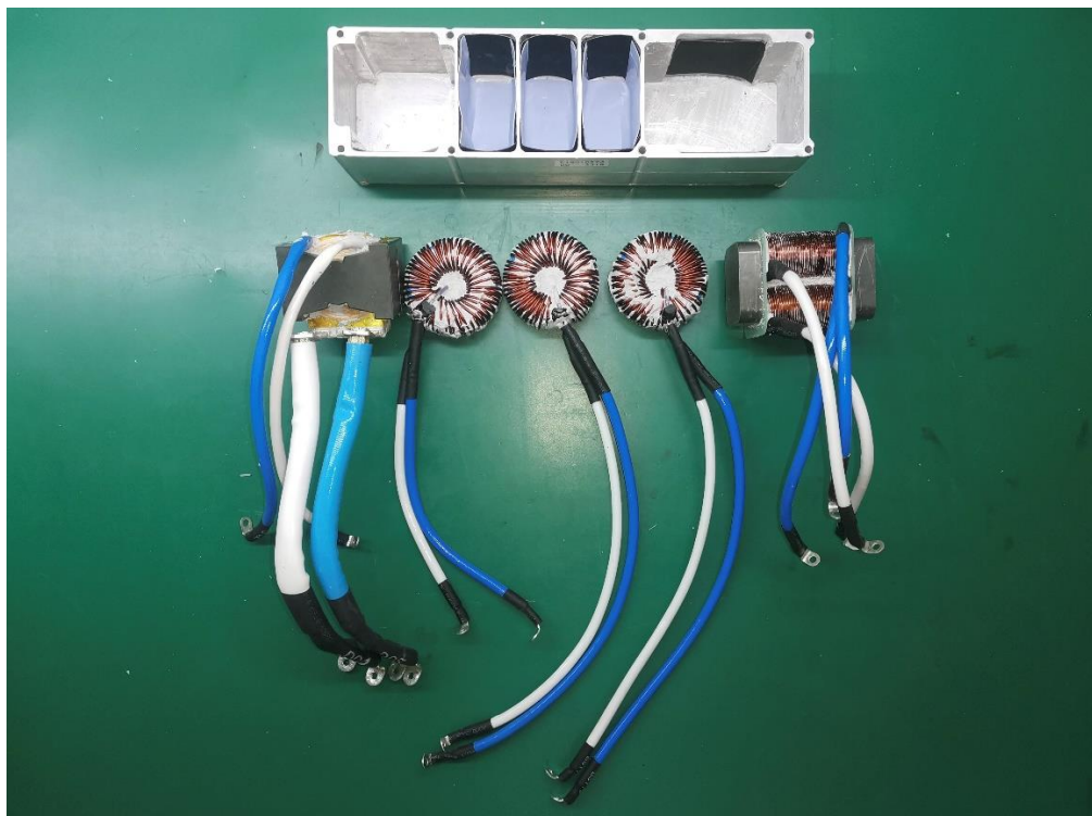
Figure 20 internal view of Transformer T17 and inductors L21~25
